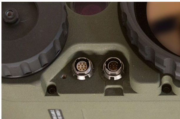
TiCAM 1000C USB connector (right)
